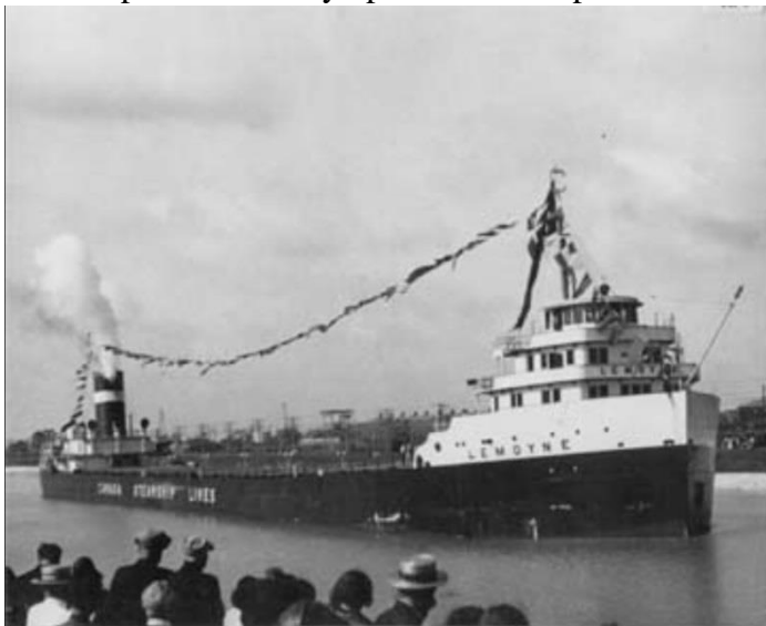
Dimensions: 621' length x 70' beam x 25.3' depth.
